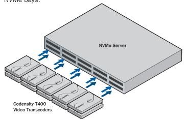
A mid-range Intel® multi-core 1U server with 10x NVMe bays can host 10x T400 transcoder modules supporting 80x simultaneous 1080p @ 30 fps real-time transcoding sessions.
