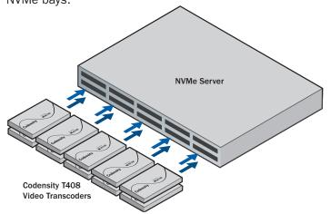
A mid-range Intel® multi-core 1U server with 10x NVMe bays can host 10x T408 transcoder modules supporting 80x simultaneous 1080p @ 30 fps real-time transcoding sessions.
