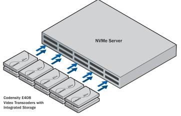
A mid-range Intel<sup>®</sup> multi-core 1U server with 10x NVMe bays can host 10x E408 transcoder modules supporting 80x simultaneous 1080p @ 30 fps real-time transcoding sessions.
